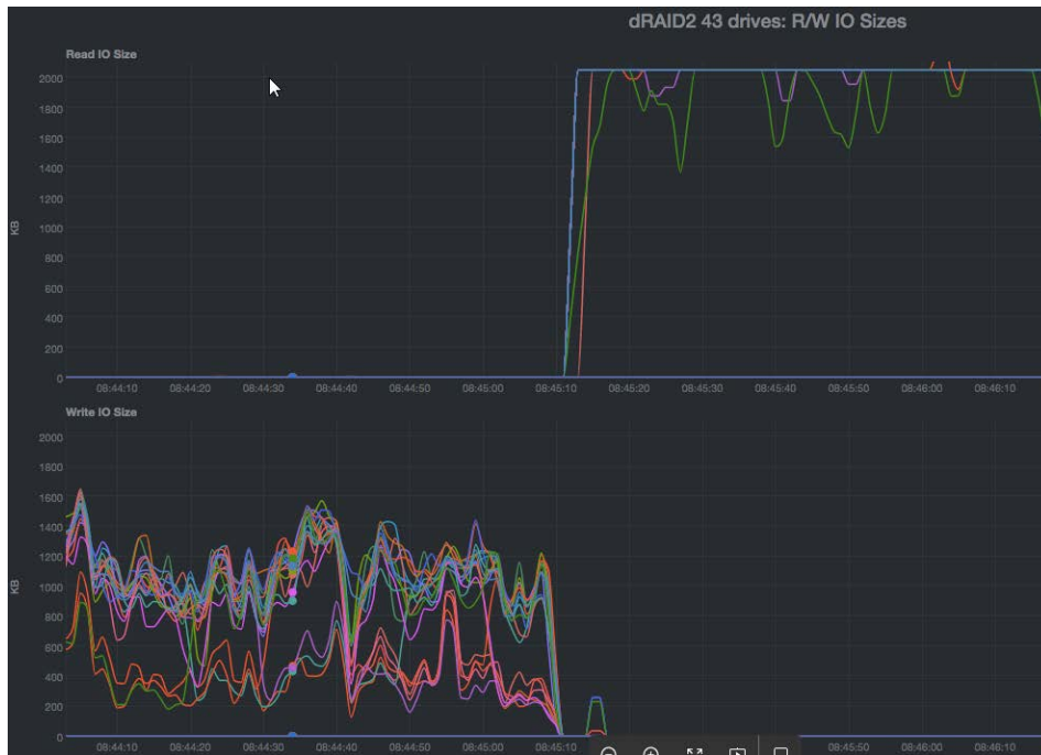
Figure 5-6. Read/Write Disk Stats for Random Workload
