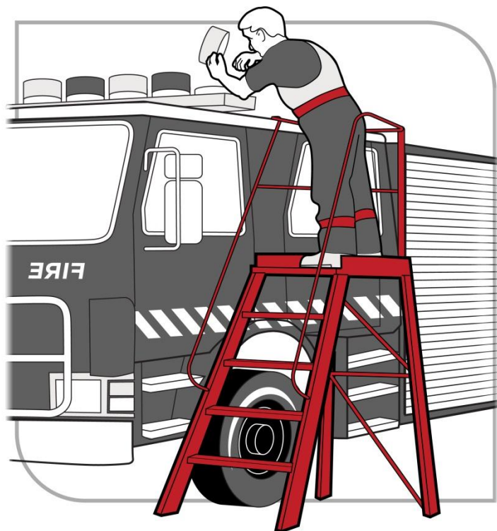
Figure 28 A step platform can provide a stable work surface
